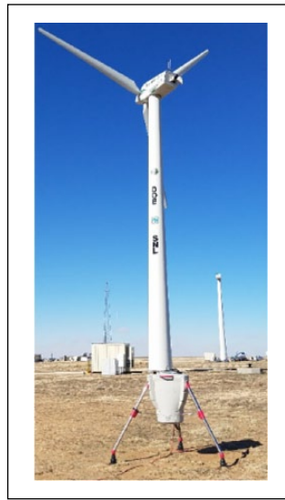
Figure 3. One of the five Pentalum Spidar LIDAR and the DTU SpinnerLidar installed in the WTGa1 nacelle.
