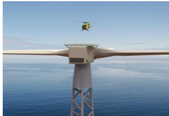
Figure 9: 2-blade offshore wind turbine (2B Energy)
