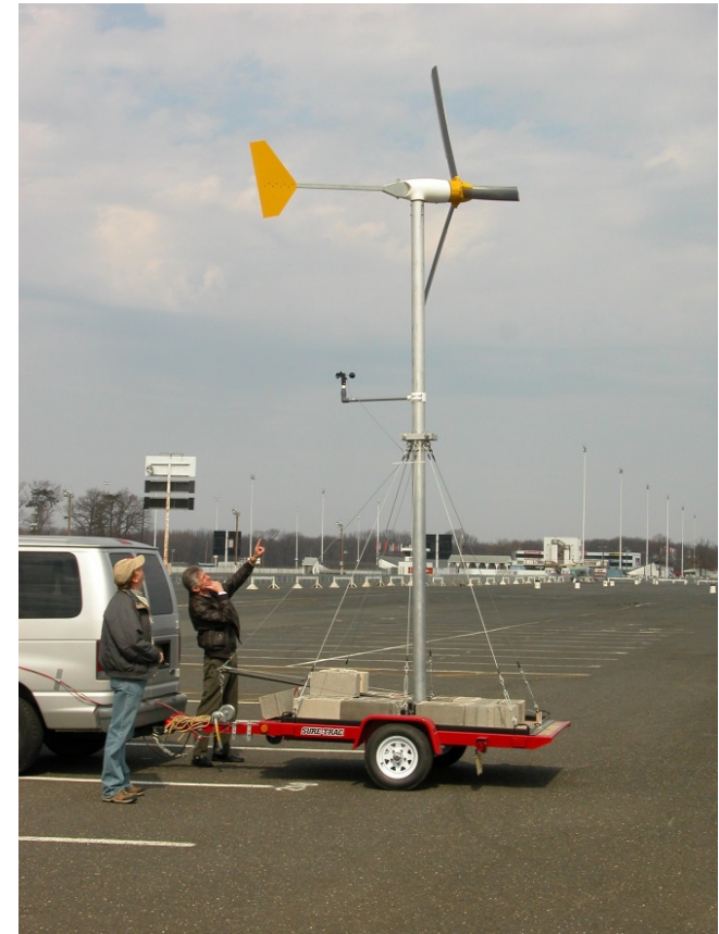
Bergey XL1 test rig with tabs installed
