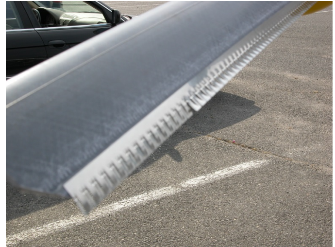
Deformable HAWT blade trailing edge
