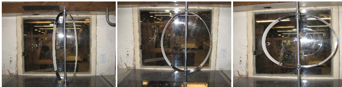
Wind tunnel model at various h/R
